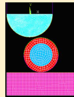
With ANSYS finite element analysis software, we are developing models of AFM indentation experiments that incorporate the heterogeneity of the sample materials by varying the mechanical properties and geometry of their finite elements. These *in silico* experiments generate virtual force-distance curves that we compare to experimental data to better understand the composition of our samples.
